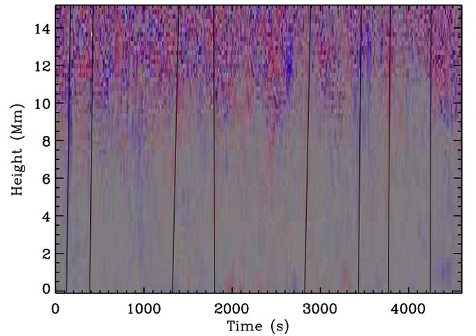
**Figure 8.** Time–distance plot of  $\delta\lambda$  fluctuations, which are proportional to  $\delta v$  fluctuations. The color scale is linear from  $\pm 0.34 \text{ \AA}$ , with red negative, blue positive, and gray zero. Black lines show the fit to tracked moving structures in the time–distance plot. The slopes of these lines indicate the speed.
