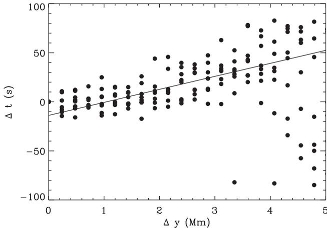
**Figure 7.** Wave travel time  $\Delta t$  versus height difference  $\Delta y$  derived from the cross-phase analysis for the intensity fluctuations at 5.9 mHz. The circles show the data derived from following the eight lowest pixels in the data set over a distance of 20 pixels. The solid line illustrates the average inferred wave speed of  $75.4 \text{ km s}^{-1}$ .
