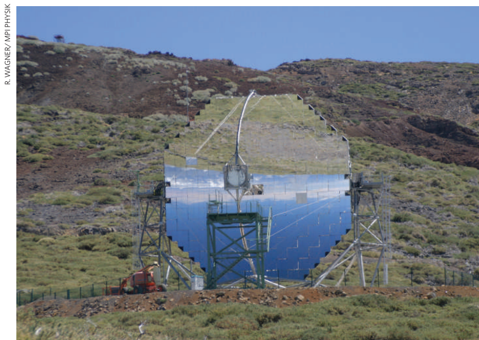
Figure 2 | Eye on the sky. The 17-metre-aperture MAGIC \gamma -ray telescope at the Roque de los Muchachos site on La Palma in the Canary Islands.
