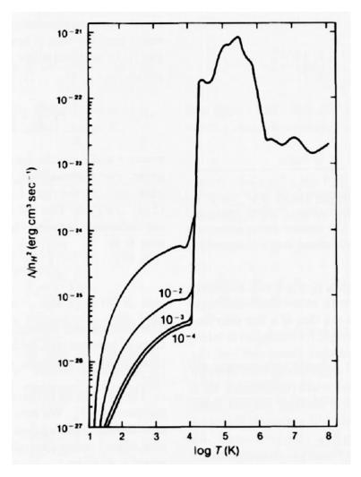
The shape of the cooling curve in different temperature ranges is due the different cooling mechanisms which are important at that temperature. For example, the sharp peak just above  $10^4$  K comes from HI cooling, while the cooling below this depends on CII and other ions with lower excitation energies. At the very highest temperatures, the emission is from Bremsstrahlung. This figure is from Spitzer (1968).
