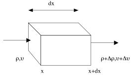
Mass conservation tells us that the change in mass  $\Delta M$  in some time  $\Delta t$  must be the mass flowing in one side minus the mass flowing out the other. In other words,
